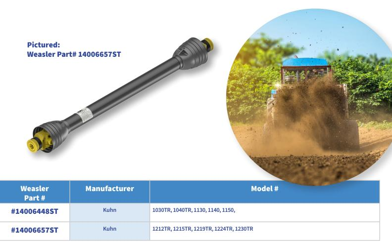
**NOTE:** Before installing verify correct end yoke and overall driveline fitment. It may be necessary to cut the driveline to length to fit your specific application. Verify the length by ensuring that sufficient overlap of the profile tubes exists in all working positions without the possibility of bottoming out. Safety decals must remain intact if driveline has been modified.
