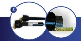
Reassemble guard halves. Both profile tubes should extend 40-mm (1.58") beyond the end of the guard tubes.
