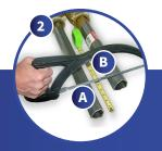
Remove guard from driveline. Separate driveline halves. Shorten guard halves (Pic. 1) and profile tube halves (Pic. 2) same as existing driveline halves or see example below.
