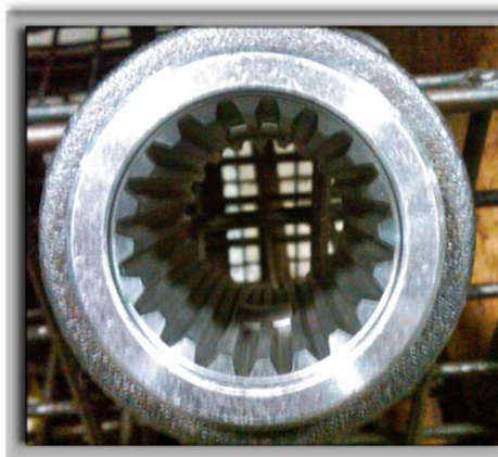
1 3/4" 20 spline - 1000 RPM "big thousand"
