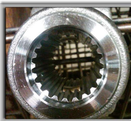
1 3/8" 21 spline - 1000 RPM "small thousand"
