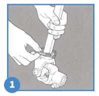
Clean and grease bushing groove before the bushing is placed in the groove. Grease any remaining bushings in guard.
