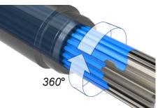
LUBRICATION TO 360° OF SHAFT SURFACE
