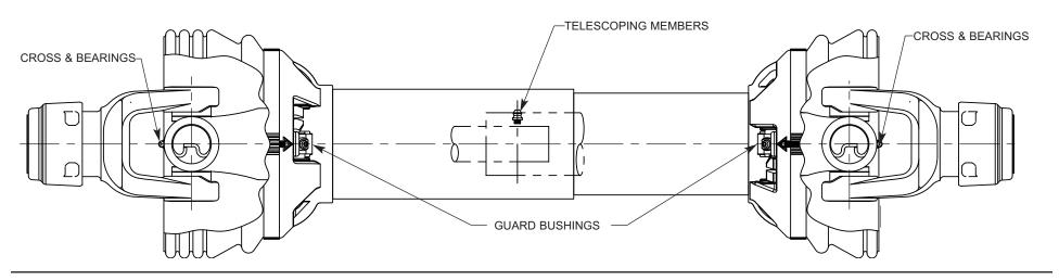
LUBRICATE ALL FITTINGS WITH A GOOD QUALITY LITHIUM SOAP COMPATIBLE E.P. GREASE MEETING THE N.L.G.I. #2 SPECIFICATIONS AND CONTAINING NO MORE THAN 1% MOLYBDENUM DISULFIDE.
