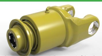
Any implement with a large rotating amount of inertia may need protection by allowing it to free wheel to a stop, independent of when the tractor PTO is stopped. This clutch will prevent the machine from driving the tractor when the PTO drive shaft has stopped. The free-running or overrunning direction is dependent on the drive direction of the PTO drive shaft. Overrunning clutches will not absorb any energy, so inertia start-up peaks must be dampened by other means.
