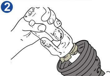
Slide guard half over drive shaft and insert bushing tabs into the opening in the guard.
