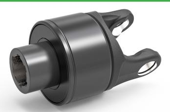
The compact automatic clutch offers a level of implement overload protection not possible with other types of clutches. The compact, efficient design disconnects the power source from the drivetrain when overload occurs, and does not reconnect until the speed is reduced. During disengagement, the patented design minimizes damaging torque spikes and heat.
