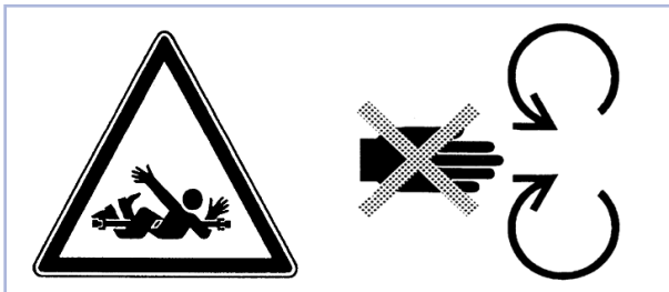
Figure B: Do not open or remove safety guard while machine or PTO shaft is running!
