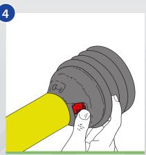
Push the Easy Lock clip into position. The bearing and guard are now secured
