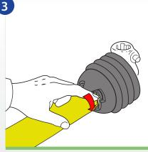
Turn the bearing until it engages into the guard
