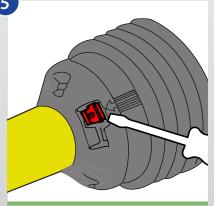
To remove guard – Use screwdriver to release Easy Lock clip. Turn the bearings to disengage from the guard and remove guard
