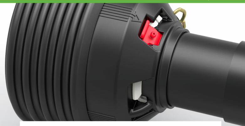
Every Weasler PTO drive line will be equipped with the user-friendly Weasler Easy Lock. This system allows for easy guard removal and replacement within seconds if servicing is required. It makes the lubrication of the joint through the Easy Lock easier
