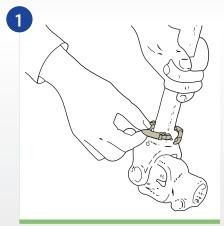
Clean and grease bearing raceway before is placed in the groove
