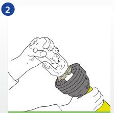
Slide guard half over PTO drive shaft insert bearing tabs into the opening
