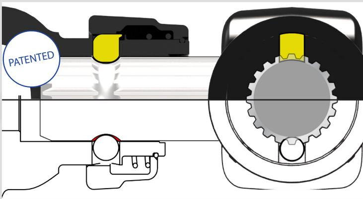
Unique Pawl Design with a compound radius to perfectly fit contour of groove. (Compared with a ball bearing)
