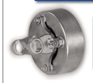
The MODULAR automatic clutch offers a level of implement overload protection not possible with other types of clutches. The efficient design disconnects the power source from the drivetrain when overload occurs, and does not reconnect until the speed is reduced. During disengagement, the patented design minimizes damaging torque spikes and heat.
