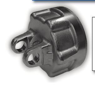
The INTEGRAL automatic clutch offers a level of implement overload protection not possible with other types of clutches. The efficient design disconnects the power source from the drivetrain when overload occurs, and does not reconnect until the speed is reduced. During disengagement, the patented design minimizes damaging torque spikes and heat.
