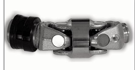
The constant velocity universal joint (CV) allows smooth machine operation through a broad range of motion. These joints allow the machine to be designed with the input shaft in the best operating position and yet allow the operator to maneuver as needed. The CV delivers constant power by self-canceling torque and speed fluctuations typically found in single cardan-type universal joints.
